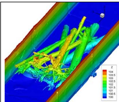
Figure 4. 3D numerical model simulation of log jam hydraulics.
