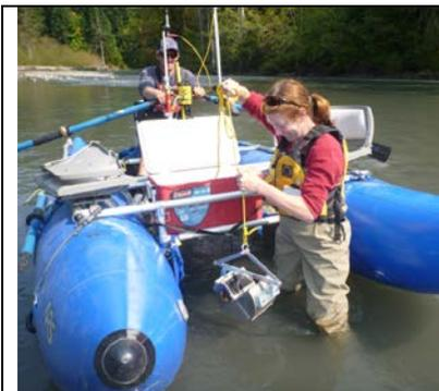
Figure 1. Sediment sampling on the Elwha River, WA.
