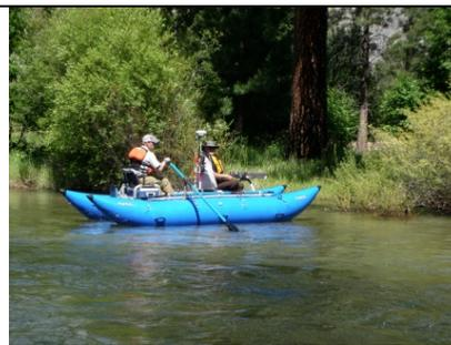
Figure 2. River channel surveys from a raft using GPS and depth sounder.
