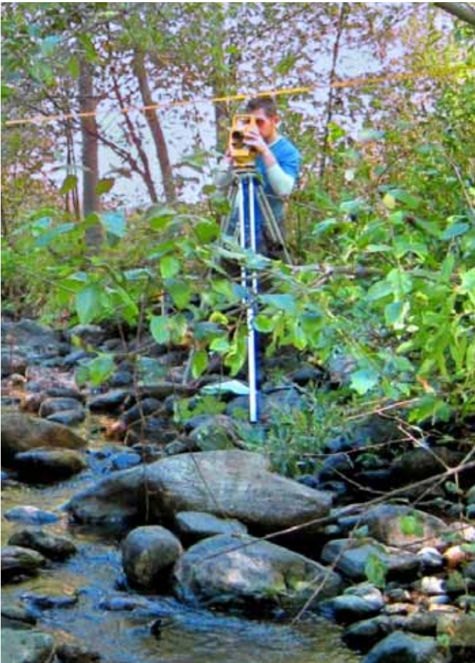
Wes using a total station to shoot a cross section of Rush Creek near Weaverville, California.
