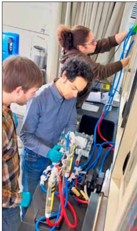
Constructing a bench-scale direct contact membrane distillation system. From left to right: Ryan Gustafson, Dr. Achilli, and Joanna Murphy.
