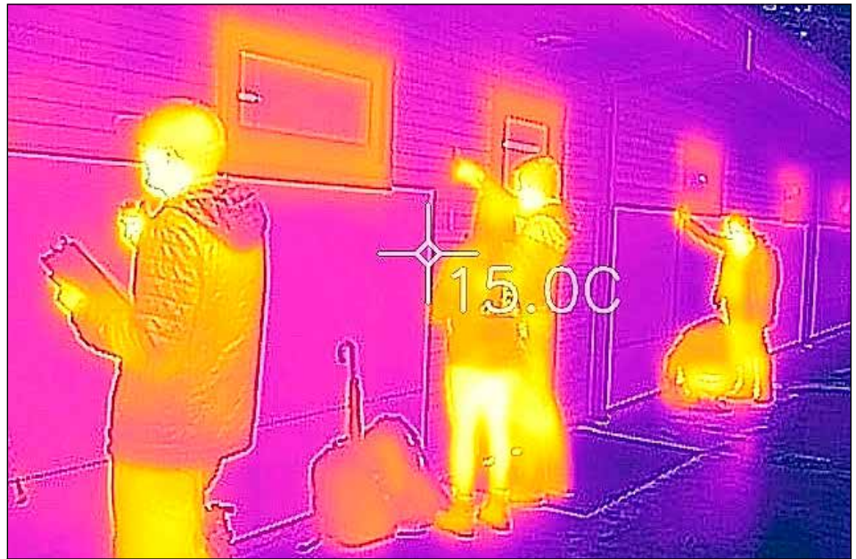
ERE Students in Professor Peter Alstone’s ENGR 473 “Building Energy Analysis” laboratory conducting a thermal analysis of the SERC West Wing in Spring 2019. The image was taken with an IR (infrared) camera.
