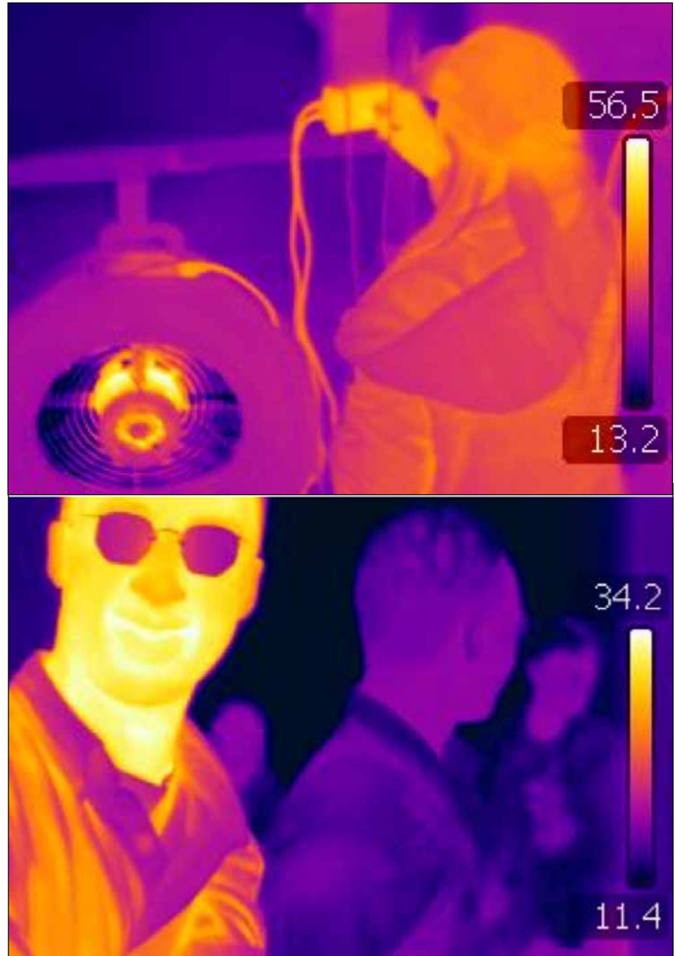
A pair of thermal images captured during a Building Energy Analysis lab exercise involving heat transfer in buildings. TOP: a student operating a blower door that allows measurements of air leaks in a building. BOTTOM: a smiling student illustrates how infrared light does not pass through eyeglasses, but can reflect like a mirror off of a nearby window. Photos by P. Alstone
